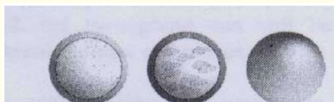
Figure 1: From left to right: Microcapsules with solution as core, Microcapsule with cell suspension as core, Microsphere with matrix encapsulated active agent.
