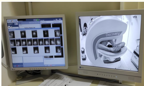
Figure 5: Semiconductor cardiac gamma camera “Discovery CZT 530c” by GE (Central Military Hospital – University Hospital Ružomberok).
