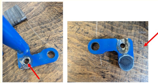
Figure 14: Damaged small impact bars at L-shaped side part.
