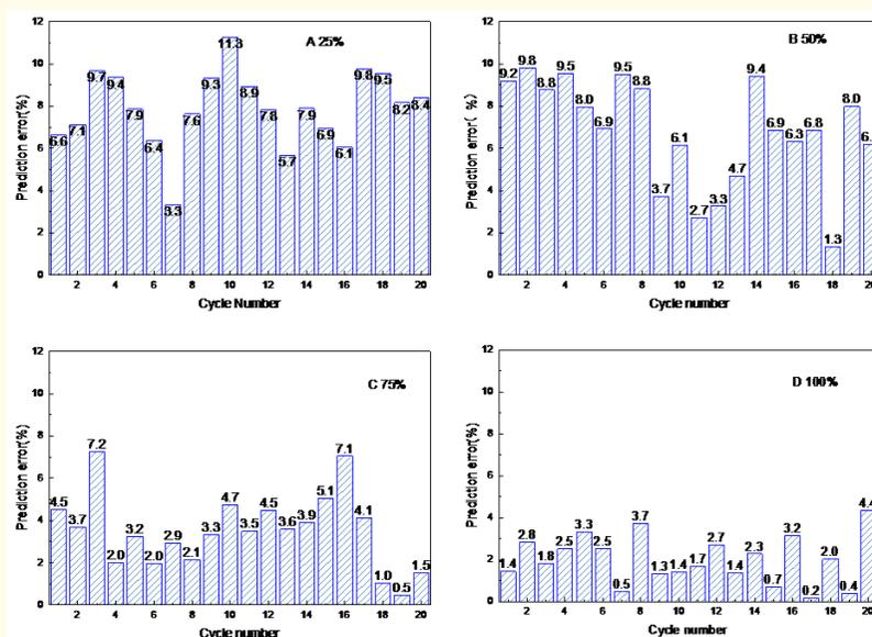
Figure 8: Prediction error of multi-cycle combustion parameters under typical operating conditions.
