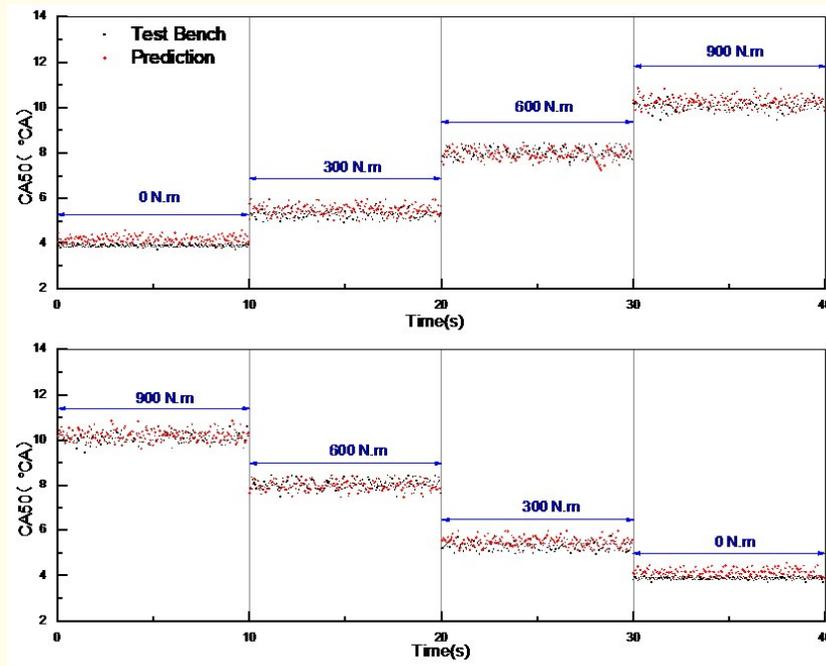
Figure 10: Comparison of real-time verification results under different steady working conditions.
