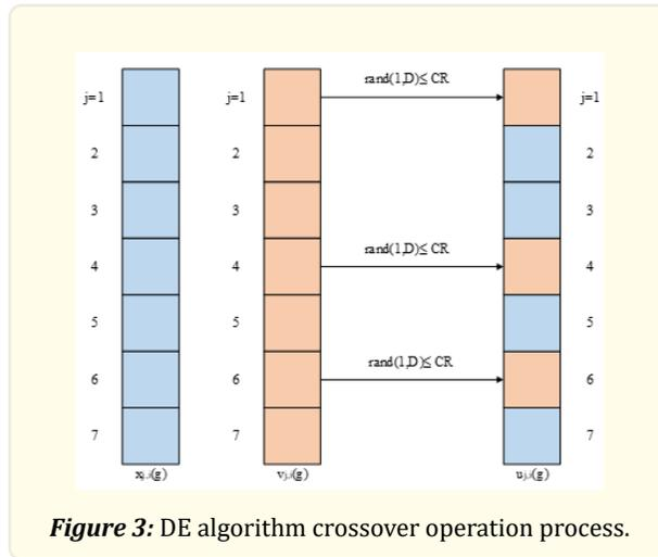
Figure 3: DE algorithm crossover operation process.
