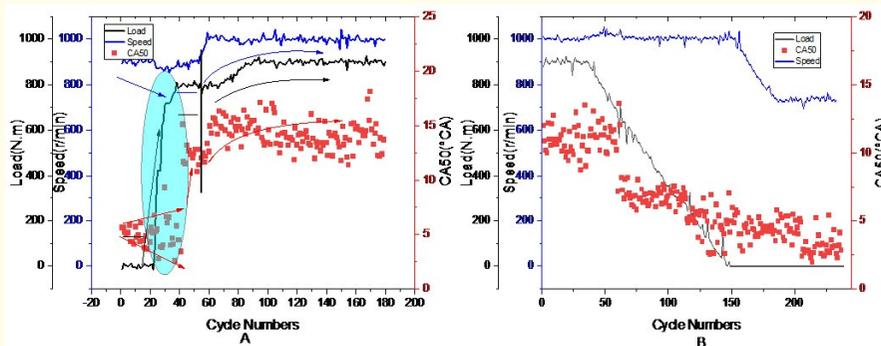
Figure 11: Transient switching condition CA50 tracking calculation.
