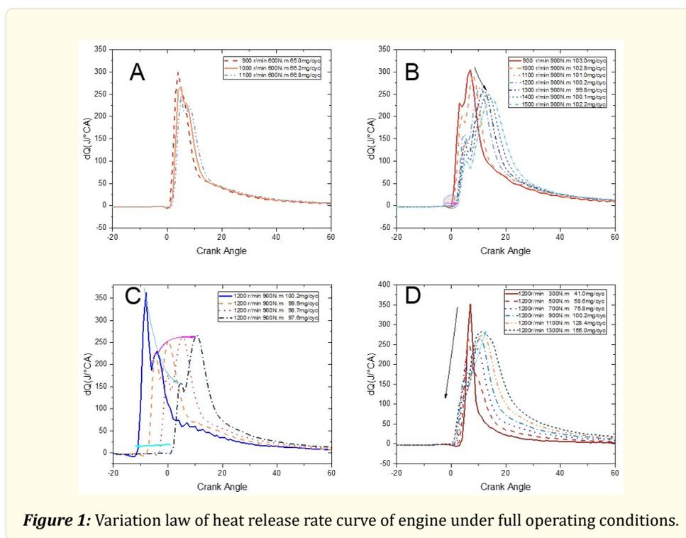
**Figure 1:** Variation law of heat release rate curve of engine under full operating conditions.
