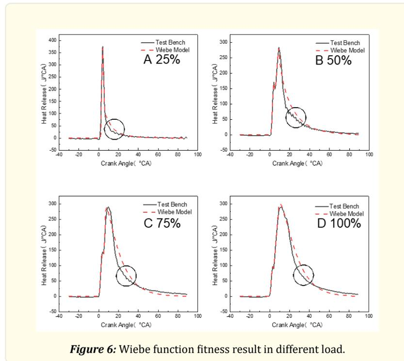
Figure 6: Wiebe function fitness result in different load.
