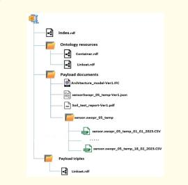
*Figure 4:* ICDD structure for verification use case.
