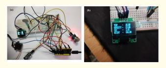
Figure 5: (a) Connection of Components in the storage monitoring system. (b) Display of Output values in the food grain monitoring system.
