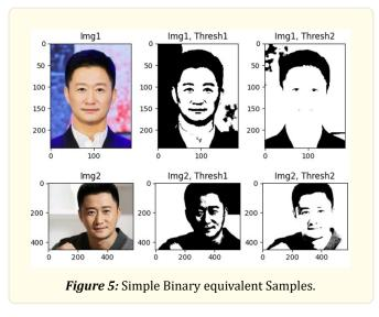
The fundamental principle of Otsu's thresholding method involves computing the between-class variance for every feasible threshold value. This approach can be decomposed into the steps listed in Table 2.
