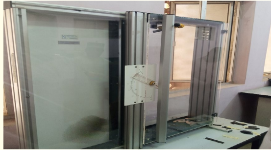
Plate III: Impact Strength Testing on Sample Composite(s).
