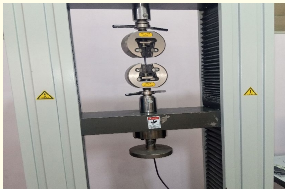
Plate II: Test Sample undergoing Tensile property test.
