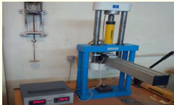
Plate IV: Specimen tested for bending modulus in 3 bending.
