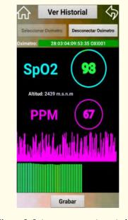
*Figure 9:* Oximeter connection window, with SpO<sub>2</sub> and PPM indicators.
