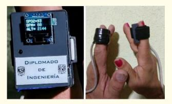
*Figure 4:* Design and manufacture of housing and thimble.
